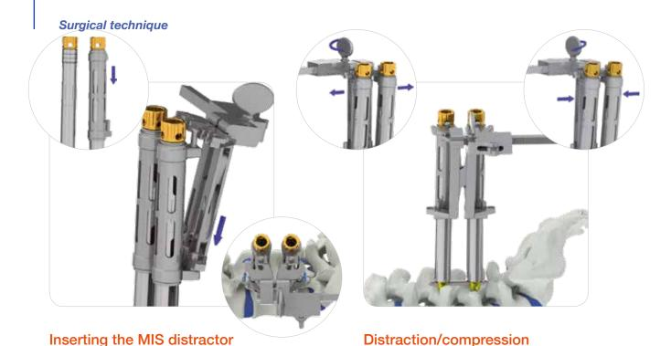
To distract/compress the vertebrae, the sleeves of the MIS distractor are guided over the head holder. In this process, the pins fixed to the sides of the sleeves are pointing upwards. Then these are pushed into the holes of the distraction unit and locked at the upper connection. Both locking plates can be opened to release the sleeves.
